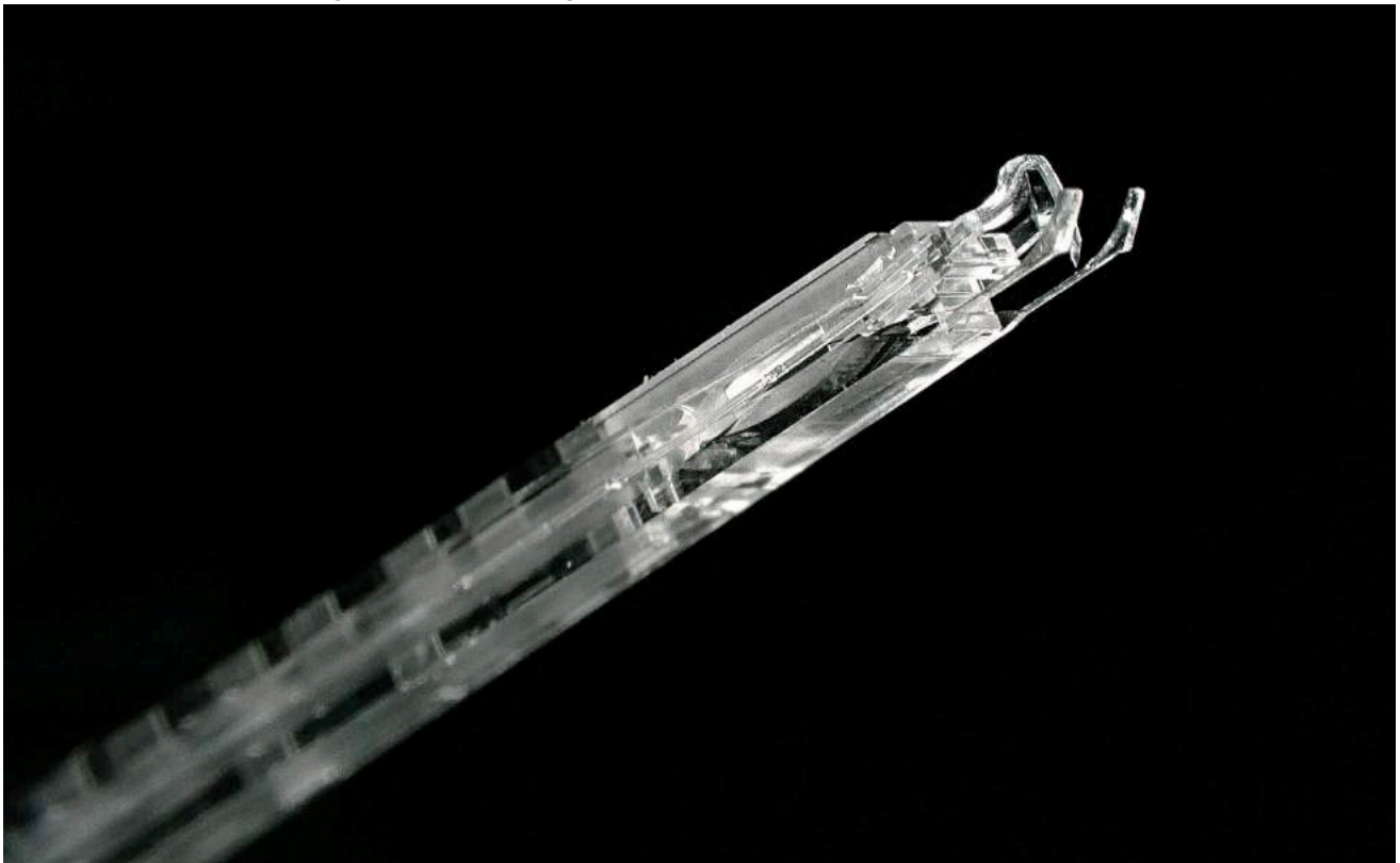
Figure 1 : SPOT femto laser-printed safe puncture tool for vitro-retinal vein cannulation
