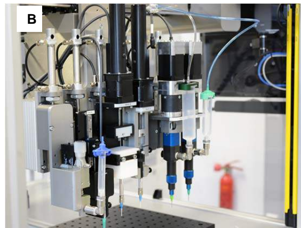
Figure 1: A: Structure of a lateral flow assay printed in a paper package; B: Multi-material 3D-Bioprinter using up to six print heads
