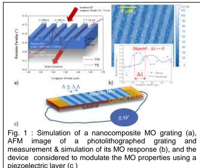
Fig. 1 : Simulation of a nanocomposite MO grating (a), AFM image of a photolithographed grating and measurement & simulation of its MO response (b), and the device considered to modulate the MO properties using a piezoelectric layer (c)
